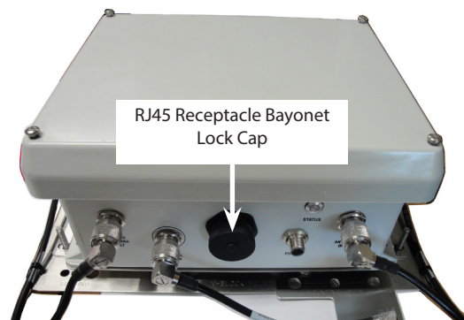
Figure 25: RJ45 receptacle bayonet lock cap (LAN with power shown.)
