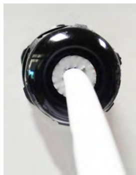
Figure 41: Gray seal after dome nut is tightened
