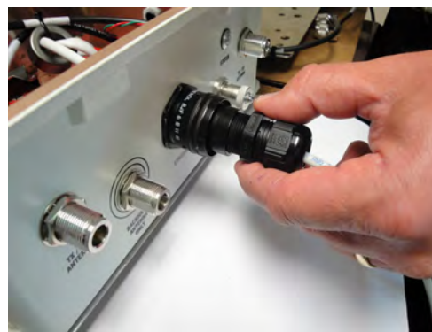
Figure 39: Tighten the cable gland nut
