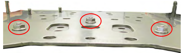
Figure 50: Remove antenna mounting bracket locknuts
