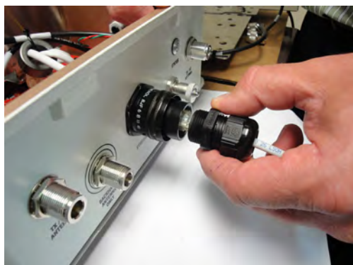
Figure 38: Screw cable gland onto metal housing
