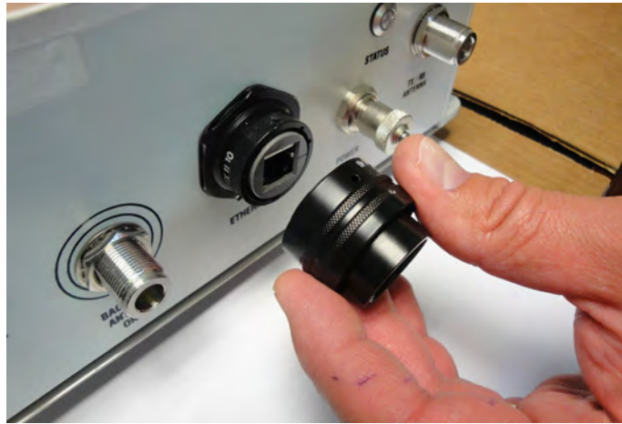
Figure 33: Remove bayonet lock cap
