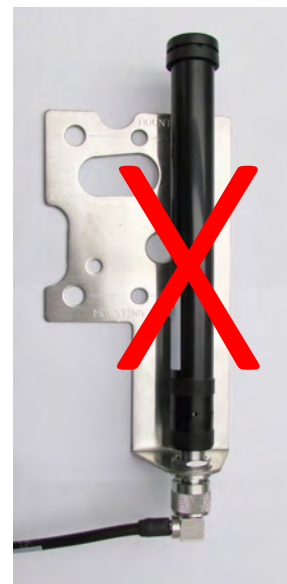
Incorrect Antenna Mount
