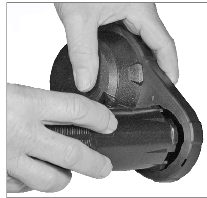
Figure 53: Pull endpoint away from base
