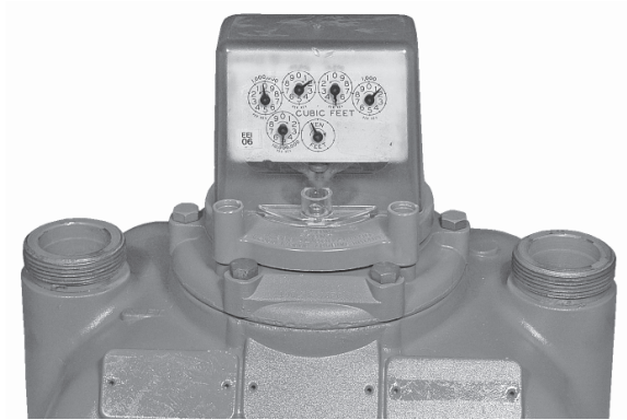
American Commercial Diaphragm and Turbine Meter with Red Security Seals
