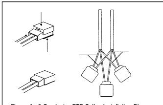
Figure 4. 3 Conductor RTR Splice Installation Diagram
