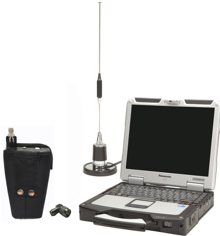
Figure 1: USB-powered mobile transceiver, magnetic mount antenna and Panasonic Toughbook
