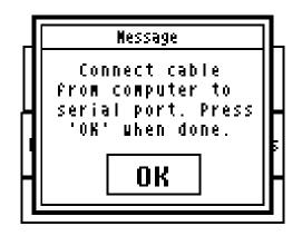
When you do this and press the Continue button, the serial communications process begins and the route is transferred from the Route Management software to The Portable Interrogator 400. As the route is transferred, you will see the screen update showing the number of bytes of information that have been successfully transferred.
