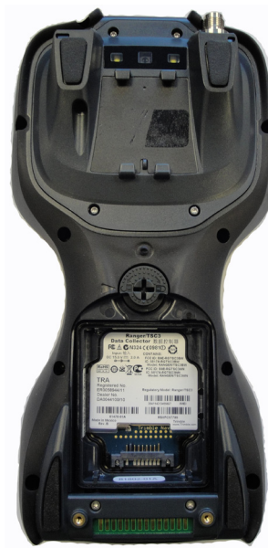
Figure 2: Inside Battery Compartment of Handheld
