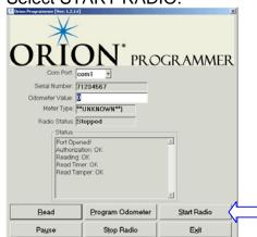
On the laptop, move the cursor to the Odometer Value box. Select it.
