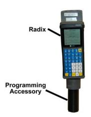
**NOTE:** Verify the IR port (the oval shaped hole on the bottom of the Badger-Radix unit) is over the opening of the Programming Accessory.
