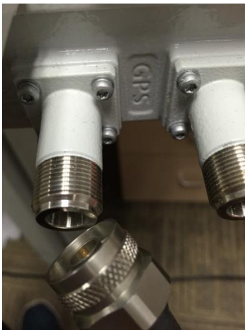
Figure 3-18 GPS Connector Connect to Base Station
