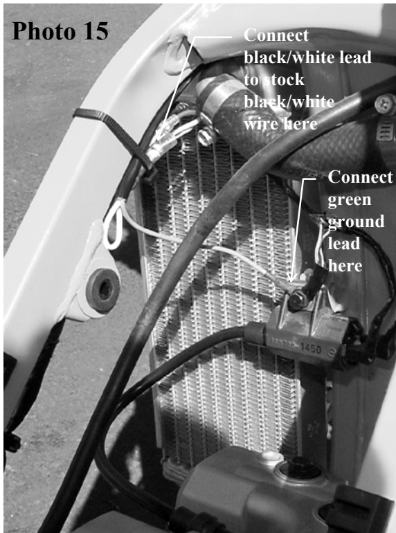
isolate the Baja Designs wiring harness from the bike's stock ignition system, and the bike will run whether or not the switch is on or the wiring is damaged.
