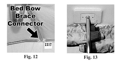
11. Inside the unit, for the bed and slideout tent set up, insert the bed bow brace at the bed bow connector. (Fig. 12) Push the bed bow outward and upward while pressing on the button farthest from the end and slip it into the bracket mounted on the roof. Release the button. (Fig. 13)
