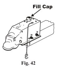
Caution: Check the fill cap before each trip for tightness. A loose cap can allow moisture to contaminate the brake fluid.
