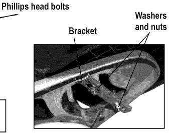
6. Secure cargo compartment with bracket, washers and nuts provided in hardware bag.
