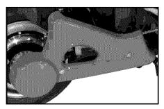
10. Attach each cover to frame using two washers and two phillips head screws.
