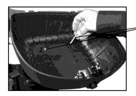
5. Place cargo compartment on rear rack of unit. Attach using two phillips head bolts.
