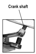
12. Attach left and right cranks to crank shaft.
