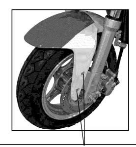
8. Attach front wheel fender to front forks with four phillips head screws, two for each side.
