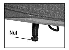
11. Remove and save nut from pedal crank shaft.
