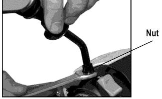
4. Insert left and right mirror into hole on handlebar and turn clockwise, secure by tightening nut.
