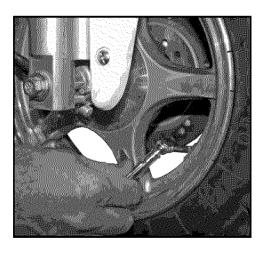
7. Fill both front and rear tires with air. Tire pressure should be se to 36psi (250kpa).
