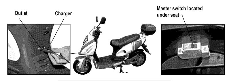
17. Charge battery before use. Turn master switch "ON". Plug charger into outlet below seat cushion. Refer to owners manual for charging times.
