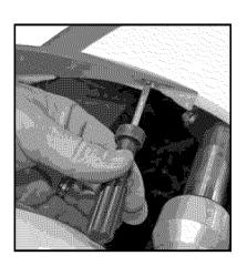
9. Align front nose piece under front panel and snap into place. Secure with two phillips head screws.
