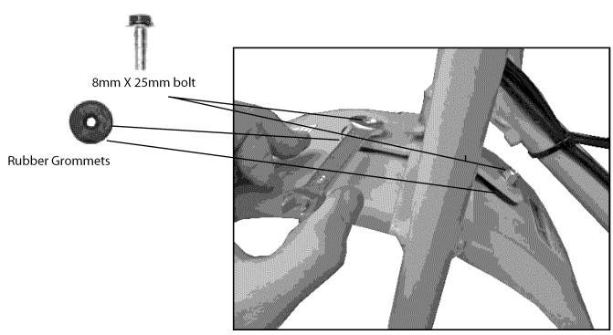
1. Install front fender. Make sure large portion of fender is over wheel. Install with rubber grommet between frame and fender. Tighten with 8mm Nuts and 8mm X 25mm bolts provided.
