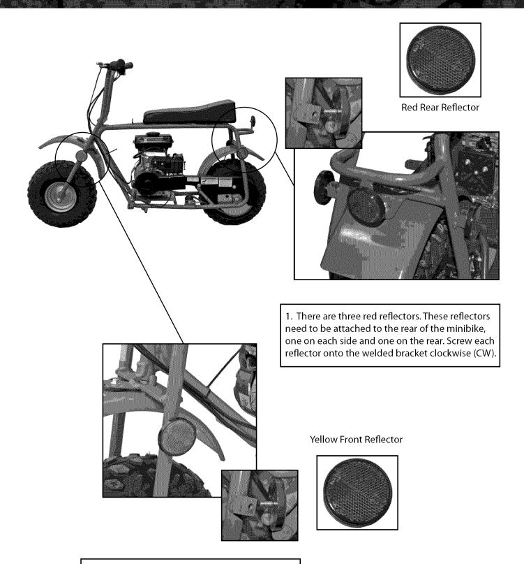
2. There are two yellow reflectors. These reflectors need to be attached to the front of the minibike, one on each side. Screw each reflector onto the welded bracket clockwise (CW).
