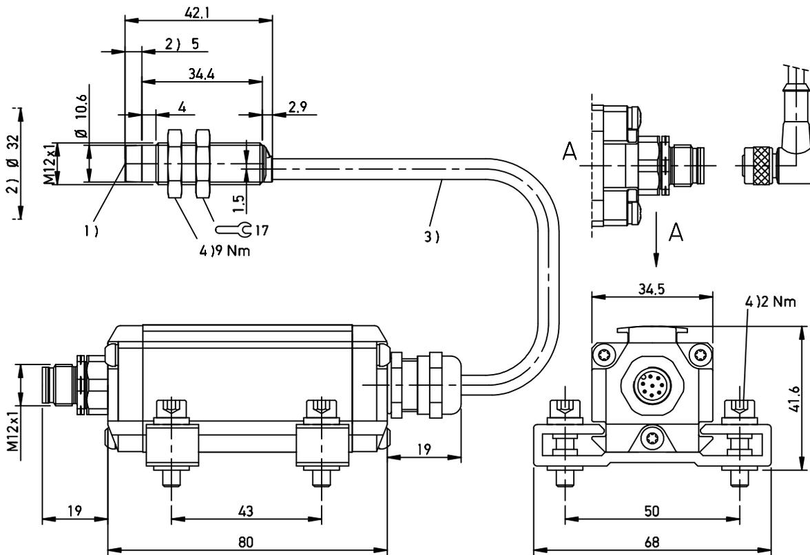
1) Active surface 2) Clear zone 3) Cable length see notes 4) Tightening torque
