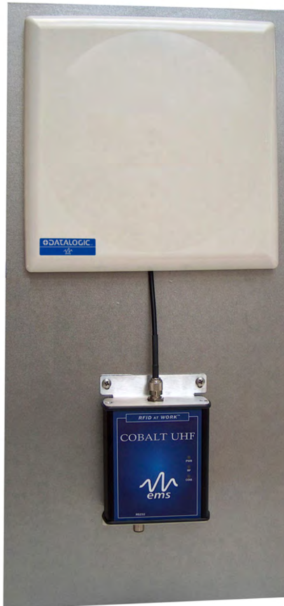
Figure 1-6: Connecting the Antenna to the Controller
