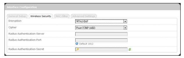
Cipher: Specifies the desired encryption protocol by clicking and selecting an option from the drop-down list:
