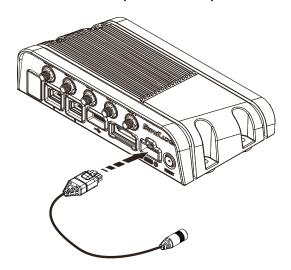
**4.** Connect the power adapter cable to either a power outlet (via the power adapter) or a 12VDC power source. The router will automatically be turned ON upon receiving power.
