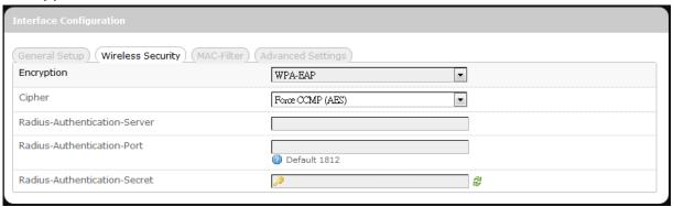
Cipher: Specifies the desired encryption protocol by clicking and selecting an option from the drop-down list:
