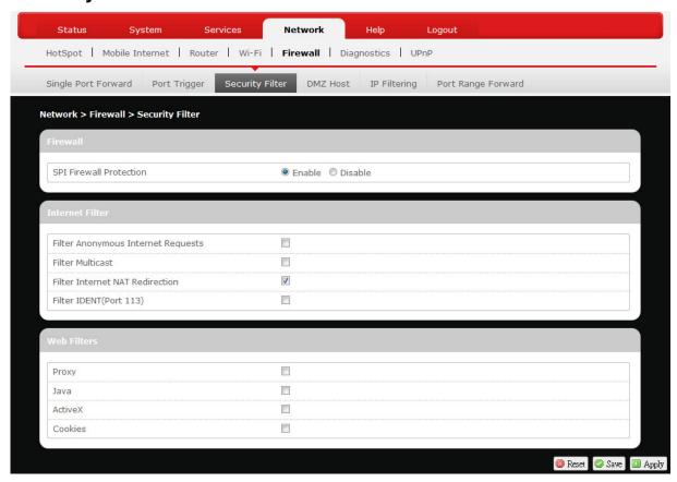
Here you can make **Firewall**, **Internet Filter**, and **Web Filters** adjustments for network security.
