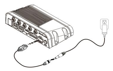
**5.** To protect the connectors from water and dust intrusion, cover all unused connectors with their respective waterproof connector protective caps.
