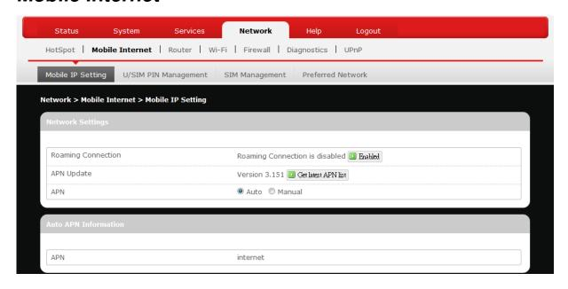
The **Mobile Internet** submenu is for setup and adjustment of mobile internet connection and furthermore has four setting tabs: **WWAN Setting**, **U/SIM PIN Management**, **SIM Management**, and **Preferred Network**.
