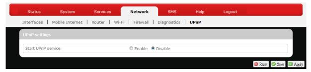
Universal Plug and Play – Allows wired and wireless network devices to discover each other and establish network services.
