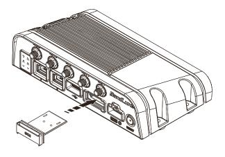
**3.** Connect the power adapter cable to the router.
