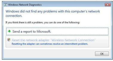
3. If you use Local Area Connection to connect the Router, please click Network and Sharing Center > Manage network connections > Local Area Connection > Diagnose, follow step 1 and the subsequent messages to repair it.
