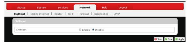
The **Hotspot** submenu is for setup and adjustment of mobile internet connection through WLAN (wireless local area network).
