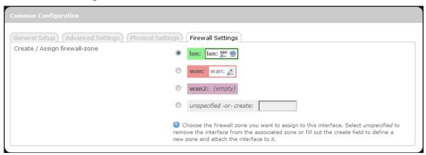
This tab is for adjustment of firewall settings.
