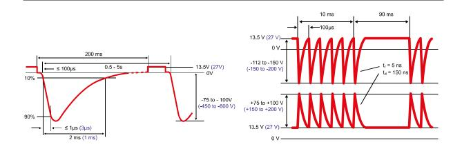
Your K530 is designed to handle large voltage swings from 9V to 32V, in case of undesirable voltage transients or brown-outs. However, for best use and proper protection of your K530, it is necessary to regulate input voltage before feeding it to the power input of your K530.
