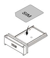
b) Insert your loaded SIM card tray into the slot on the router.
