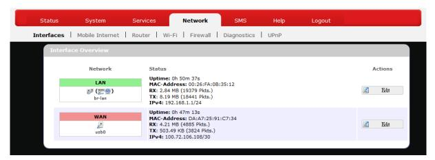
The **Interfaces** submenu allows interface configurations of different networks connected to this router. The configuration items are the same for each network with different default settings.
