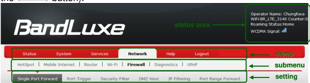
Note: If SIM Card's PIN verification is needed, select Network > Mobile Internet > U/SIM PIN Management.
