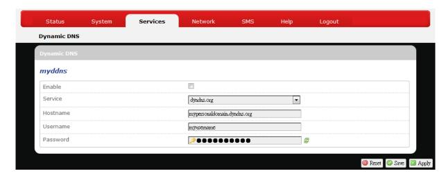
The **Services** menu hosts configuration options for DDNS (Dynamic Domain Name Service), which is a system that allows the domain name data held in a name server to be updated in real time. It allows an Internet domain name to be assigned to a computer with a varying (dynamic) IP address. Before you can use this feature, you need to sign up for DDNS with a DDNS provider, www.dyndns.org or www.TZO.com.
