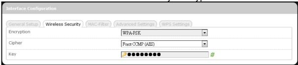
Cipher: Specify the desired encryption protocol by clicking and selecting an option from the drop-down list:
