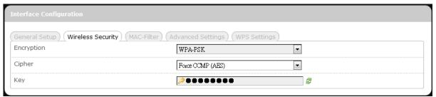
This router supports wireless data encryption, a must for wireless data security. The Wireless Security Interface Configuration items will change according to the chosen encryption method.
