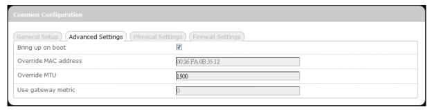
This tab is for advanced users to make detailed configurations of protocol-related settings. Actual configuration items will vary according to the protocol chosen in the tab item *General Setup*.
