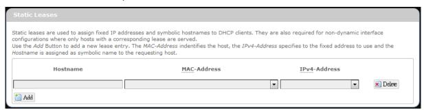
Enter the desired hostname. Choose the desired MAC address and IPv4-Address (click and select a rule from the drop-down list; if "--Custom--" is selected, the drop-down list will change to a text box to allow you to enter your custom address).
