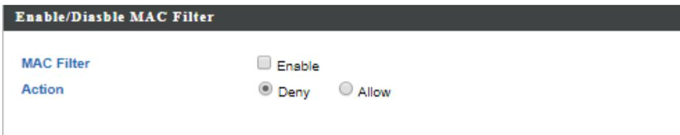
This section allows users to filter wireless connections by MAC address.
