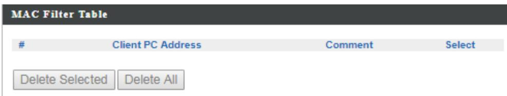
This section allows users to manage MAC address filtering entries. All MAC address filtering entries you have created will be displayed in this table.
