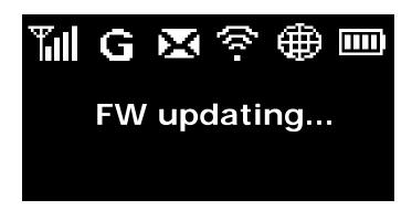
If the firmware version on the device is being updated via the Web interface, the screen informs the user of the process.
