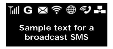
When a broadcast SMS is received, it is displayed on the screen, in ticker format if necessary. Press the WPS button to clear the message.
