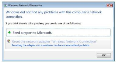
3. If you use Local Area Connection to connect the Router, please click Network and Sharing Center > Manage network connections > Local Area Connection > Diagnose, do the step 1 and following the message to repair it.
