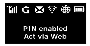
If the user has enabled the PIN security protection on the SIM card, the screen directs the user to access **4G LTE > PIN Verification** via the web
