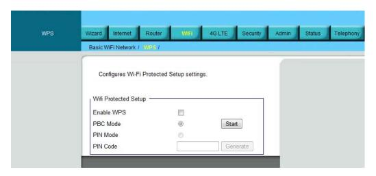
Wi-Fi Protected Setup (WPS) is a standard designed to easily setup and automatically configure secure Wi-Fi networks between two WPS supported devices. If the client PC supports WPS, the WPS feature can be a user-friendly and simple process to get your Wi-Fi network up and running.
