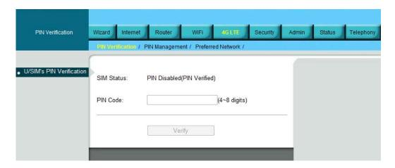
If your SIM card PIN protection is enabled, you must enter the PIN code for verification. Enter the code in the PIN Code field, and click **Verify**.
