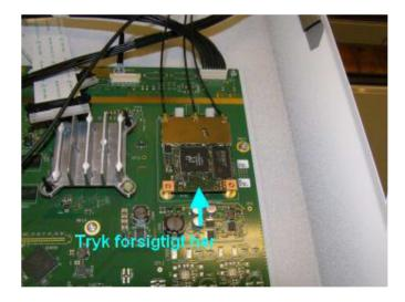
Fasten the WLAN-module with 2 2.5 mm nuts End of Procedure
