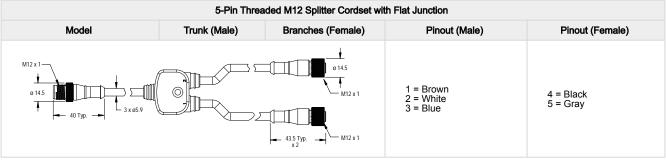
**NOTE:** The splitter in the PRO-KIT has two male and one female connectors. The CSB-M1251M1251B splitter has one male and two female connectors. Use the CSB-M1251M1251B to connect the sensor to power and a one of the Banner Pro lights with the Pulse Pro output.
