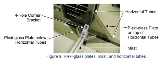
4 Attach horizontal-plexi-glass assembly to corner brackets on Mast subassembly using 1/4-20 bolts, washers, and nuts.
