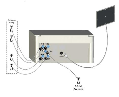
Figure 18: Antenna and solar panel connections on SAM.
