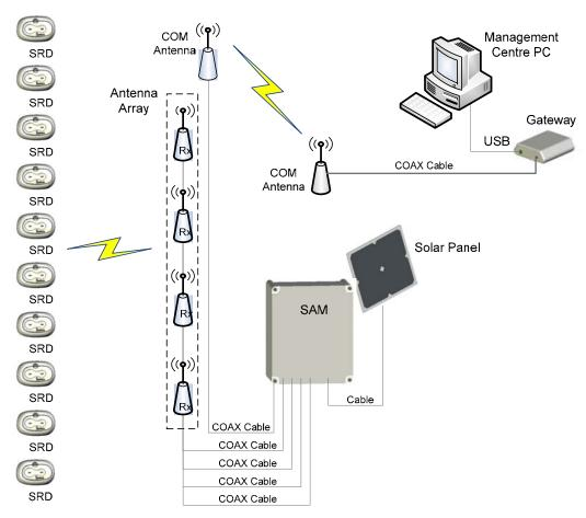
The following diagram illustrates the BarMate System. A description of system components follows.
