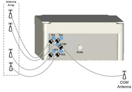
Figure 17: Antenna connections on the bottom of the SAM.
