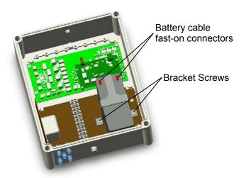
Figure 14: Battery installed in SAM.
