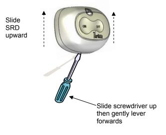
Figure 27: Disconnecting an SRD.
