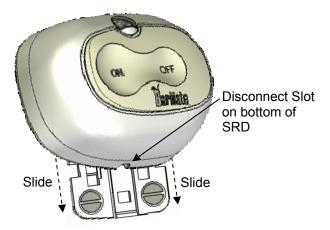
Figure 24: Sliding the SRD onto the mounting bracket.
