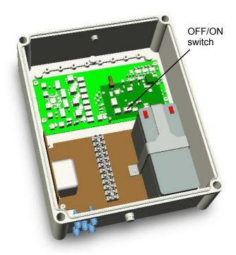
Figure 15: On/Off switch inside SAM.
