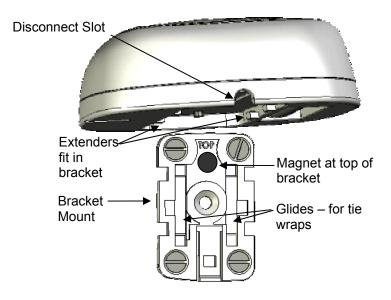
Figure 23: Connecting the SRD to its mounting bracket.
