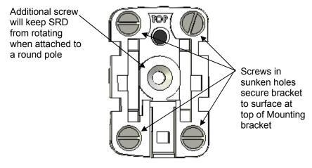
Figure 22: SRD mounting bracket and screws.
