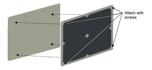
Figure 4: Solar panel and large panel mount.
