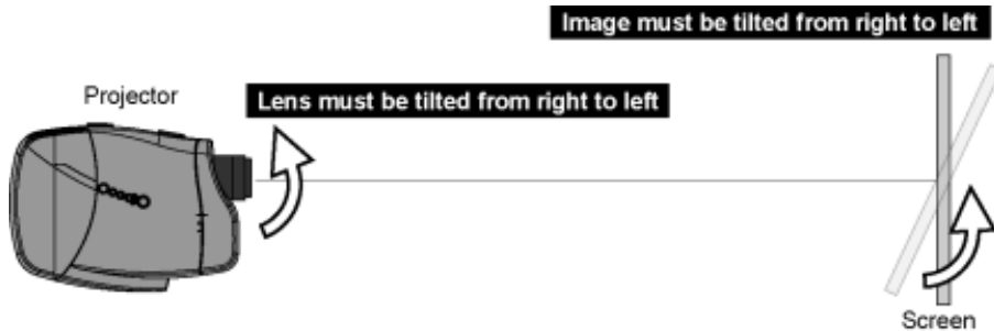
Image B-8 Lens must be tilted from right to left.
