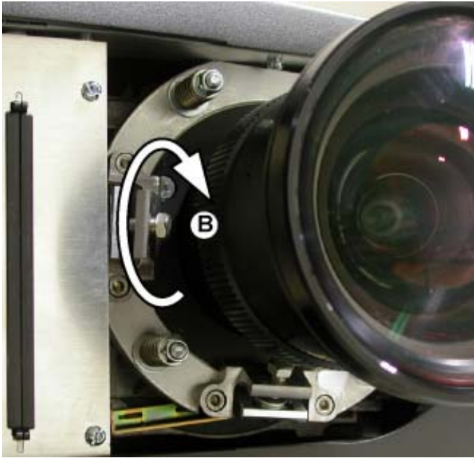
Image B-9 Screw bolt B to tilt the lens from right to left.
