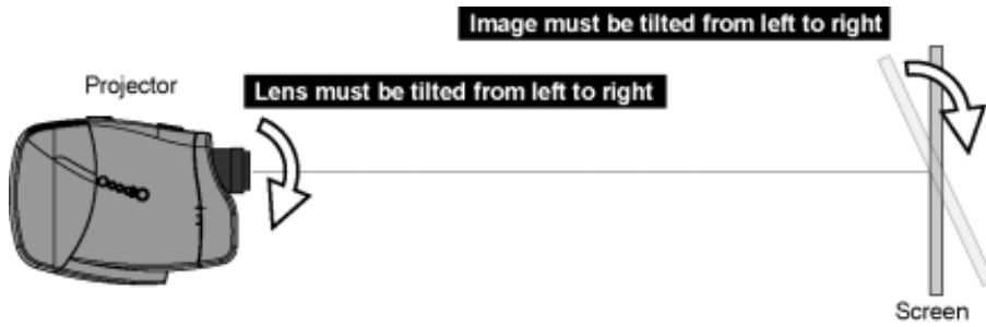
Image B-6 Lens must be tilted from left to right.
