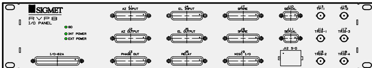
Most of the connections between the radar and the RVP8 are made using the RVP8 Connector Panel which connects to the I/O-62 by 1.8m (6 foot) cable. The panel is usually mounted on the front or the back of the same 19” EIA rack that contains the RVP8 chassis. The I/O-62 cable may be plugged into either the front or the back of the connector panel to optimize the cable run.
