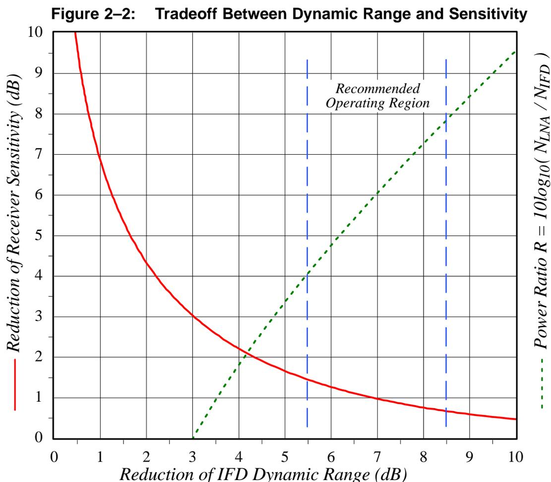
The solid red curve in Figure 2-2 shows that these two variables interact in a symmetric manner, so that any operating point  $(x,y)$  is always matched by a dual operating point at  $(y,x)$ . To understand the construction of this plot, let  $N_{IFD}$  represent the stand-alone (terminated input)
