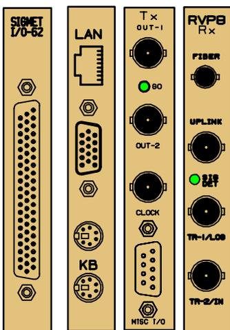
The direct connections to the RVP8 chassis are made either to the back of the unit to PCI cards (e.g., left) or to the remote connector panel. The direct connections are summarized in the table below.
