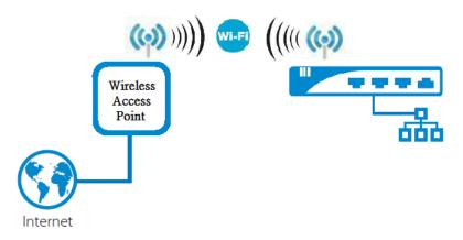
This device only supports Slave mode not supporting bridgemesh and repeater function.
