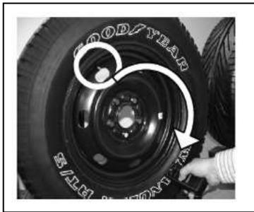
(Note with Ford Banded sensor's, the tool should be held 180° away from the stem.)
