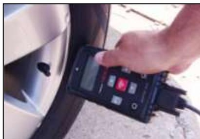
Proper tool positioning is important to insure sensor activation and decode. Place the Tech500 on the tire, at the TPMS sensor, pointed toward the sensor location as shown above.
