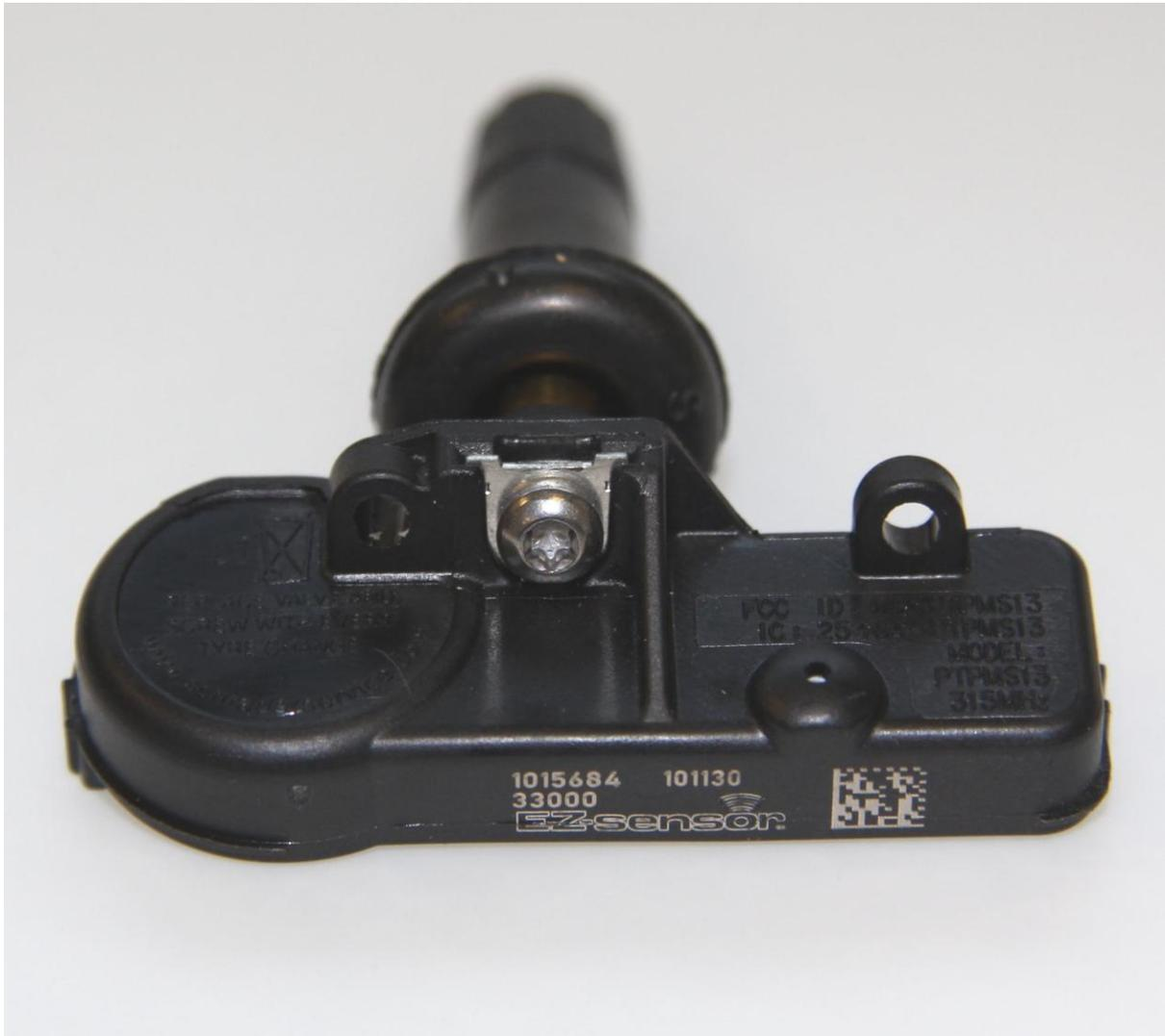
The sensor pictured above has a black body and this is a 315MHz EZSensor. The 433MHz EZSensor is grey. If the wrong part is used, the programming process will fail immediately as the PAD will identify that the wrong EZSensor is present.
