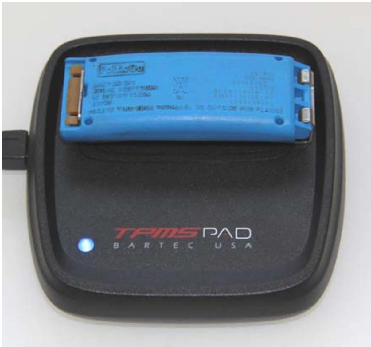
When the test process starts, the LED changes colour to indicate testing is in progress. During testing or programming, the microprocessor generates a suitable 125KHz magnetic field in order to communicate with the TPM. If the TPM is working, it responds with a radio signal which is picked up by the PAD.
