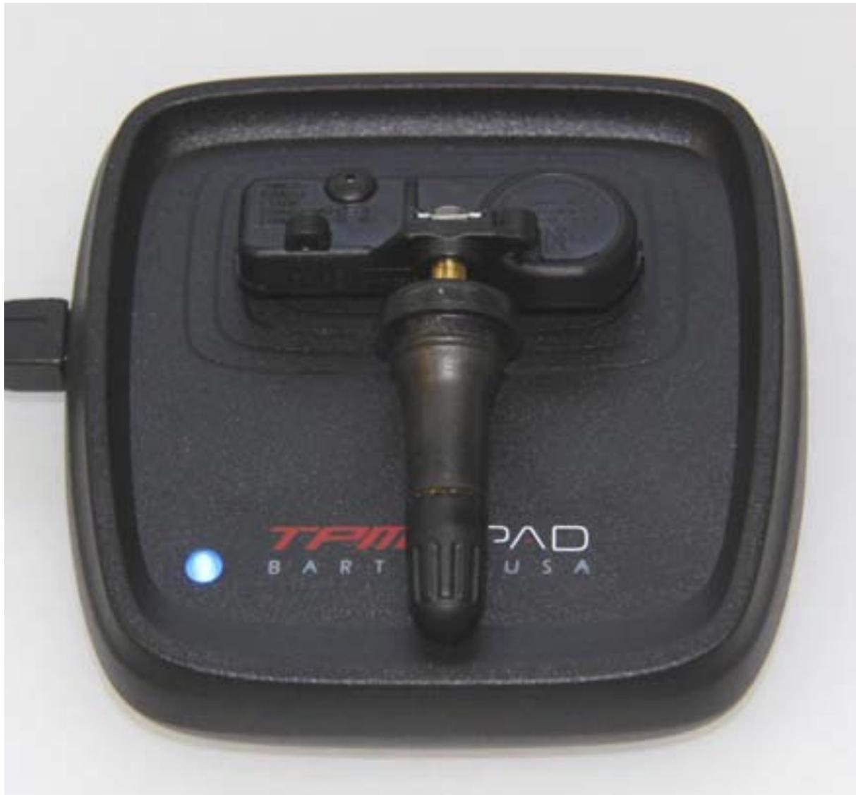
When the EZSensor program process starts, the LED changes colour to indicate programming is in progress. Programming can take up to two minutes depending on the TPM type. If the copy is successful, the LED illuminates green. If not, the LED illuminates red.
