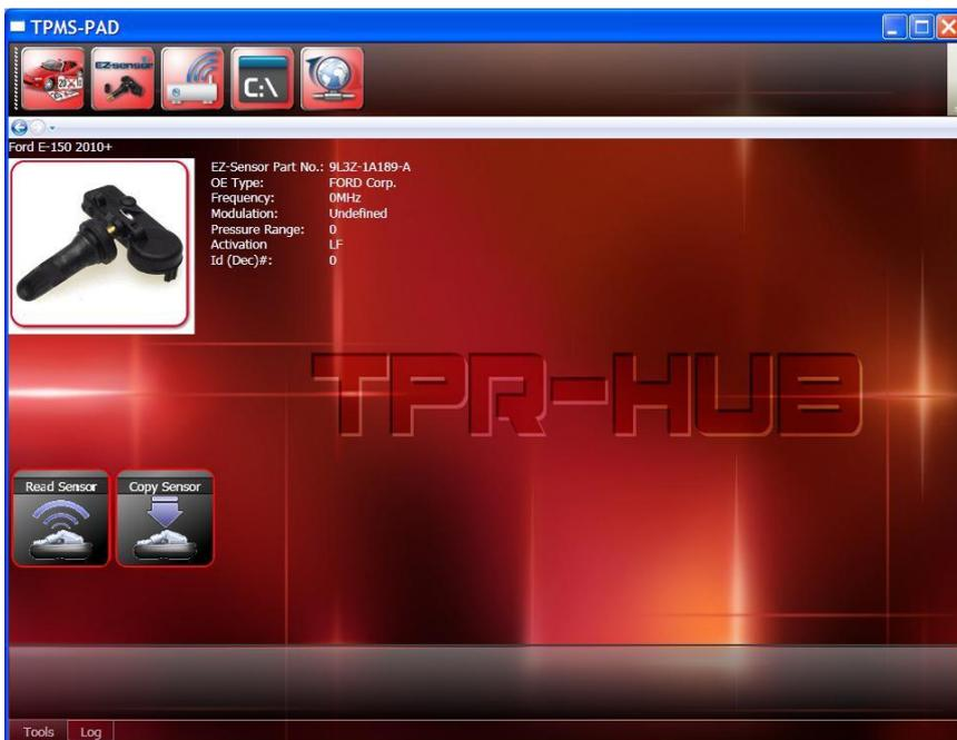
The user can then choose to test the sensor normally fitted to that vehicle by placing the sensor on the PAD and clicking on the Read Sensor button. It is important to place the sensor in the correct place on the PAD. On this vehicle, the part is a banded type and is strapped to the wheel using a steel band.
