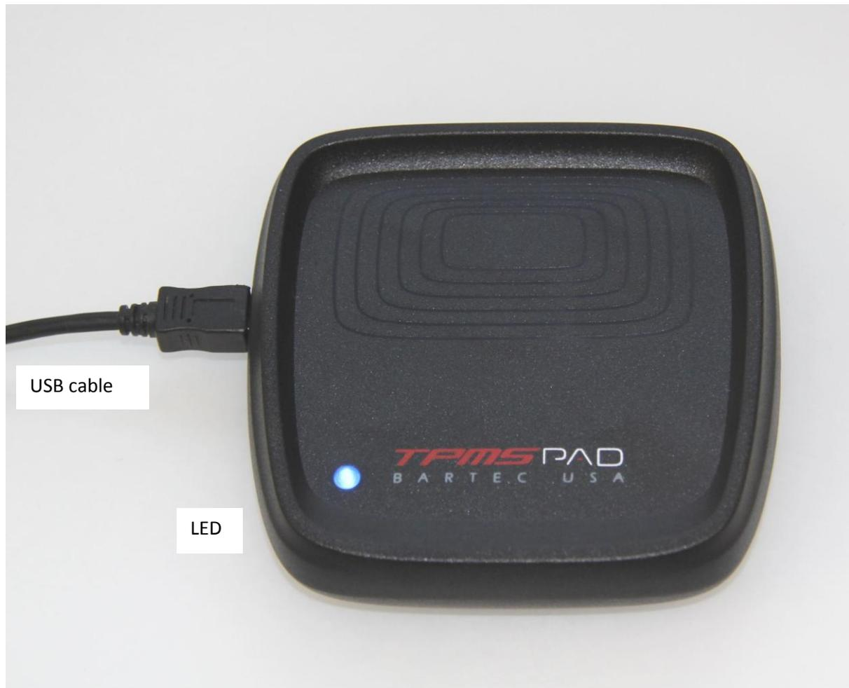
When the PC program starts, it sends a command via USB to the PAD which responds with the available vehicle makes, models and years that the PAD has in its internal data tables. The program then displays all the available vehicle makes.
