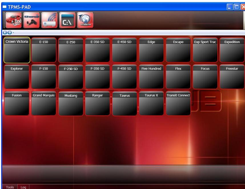
Now the E150 model is selected by clicking on the E150 button. If you make a mistake, you can click on the back button (the left arrow on the left of the screen just above the vehicle model list). In this case there are two models from different years (2007-2009 and 2010 onwards) which have different TPM sensors fitted. You will only be asked for the year if it's necessary to correctly identify the TPM fitted.
