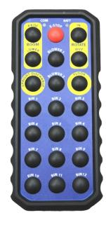
The Ranger II handheld can be equipped with different radio technologies depending on your application requirements. Currently, only one radio technology is available: Amplitude Shift Keying (ASK). The operating frequency along with other characteristics of this radio technology is outlined in the following table.
