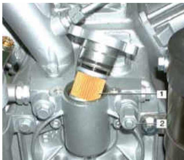
Figure 3-7 Replacing the Oil Filter
