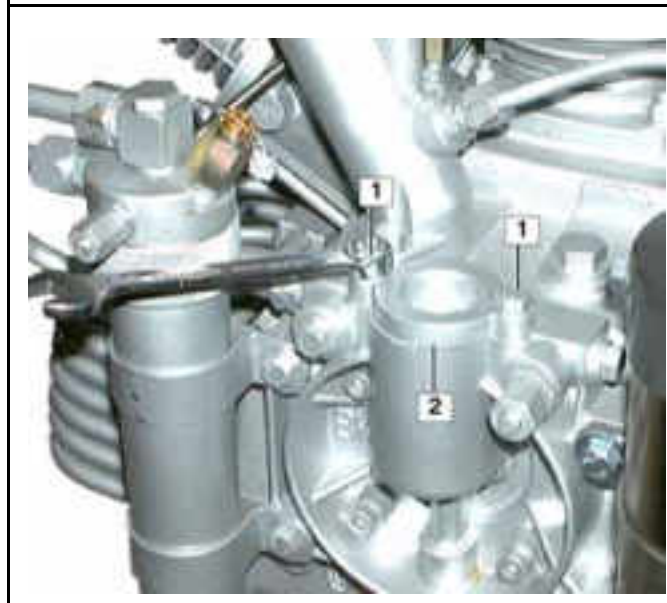
Figure 3-6 Removing the Oil Filter Cover
