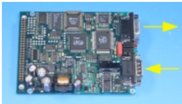
upper connector IBS-OUT, lower connector IBS-IN
