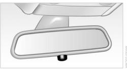
The indicator lamp below the interior rearview mirror flashes continuously: the system is armed
