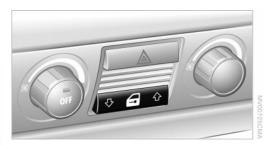
You can operate the central locking system with this button when the driver's door is closed. This unlocks 介 or locks 🕂 the doors and luggage compartment lid, but does not activate the
