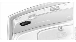
A recess has been incorporated into the inside trim on the luggage compartment lid to make it easier to pull down.
