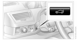
You can use this button to open the luggage compartment lid when the vehicle is stationary. This is not possible, if the luggage compartment lid has been locked separately.
