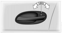
One turn of the key in the driver's door lock unlocks the driver's door only.
