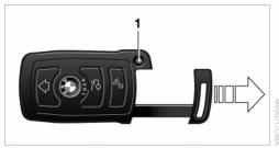
Press the button 1 to release the key.
