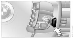
Insert the remote control unit all the way into the ignition lock. This also activates the radio mode.
