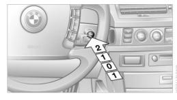
Do not depress the brake pedal until you are ready to start the engine. If you press the start/stop button while the brake pedal is depressed the engine will start immediately. ◀
