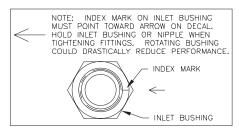
40 BCS models are equipped with a brass inlet bushing installed in the tank. Heaters equipped with this bushing are marked next to the inlet by the decal shown on the left. The purpose of this bushing is to help keep the tank bottom free of sediment by aiding tank flushing. This bushing must be located as shown on the decal to function properly. Do not allow the bushing to rotate out of position when tightening the inlet fittings.
