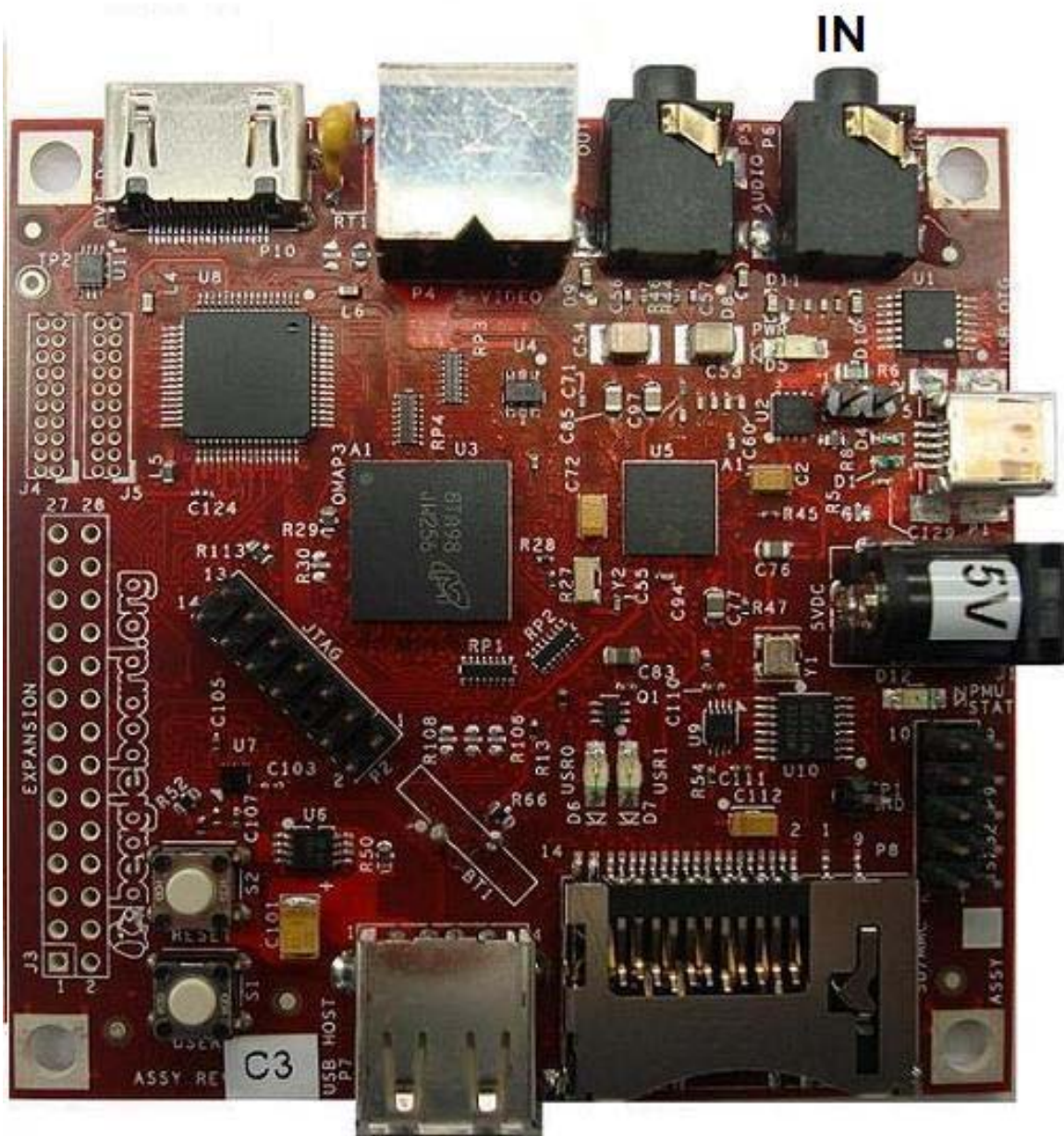
Figure 13. BeagleBoard Audio In Cable Connection
