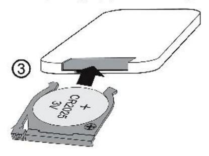
3 Slide the tray with the new battery into the battery compartment until it clicks into place.
