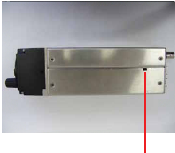
Fig. 2-2 Location of internal automatic fuse (resetable)
