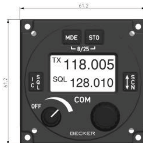
Fig. 2-3 Mounting dimensions VHF transceiver
