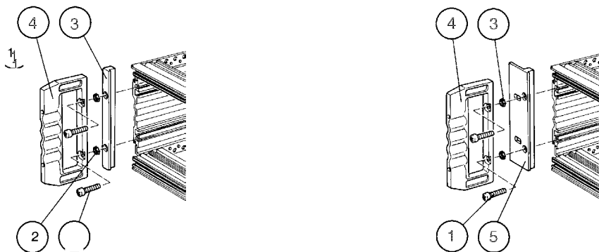
Fig. 2-1 Mechanical Installation on 19-inch adaptors
