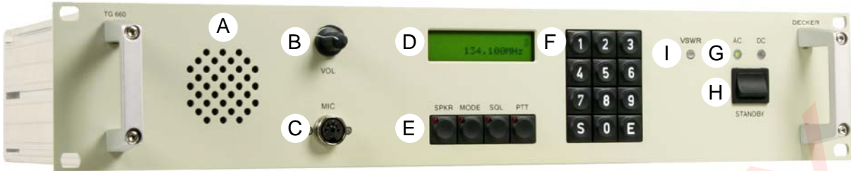
Figure 15: TG660 – Controls and Indications
