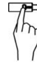
ID pairing/connect button on the top of the dongle receiver (With a LED indicator under the ID pairing/connect button)
