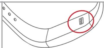
Press the charging cable into the charging port on the bottom of the wristband.
