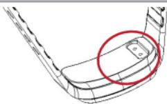
1. Press the charging cable into the charging port located on the bottom of the wristband.
