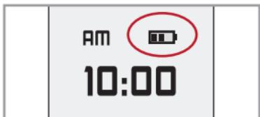
When a reminder is not present, pressing the button once will display the battery icon in the upper right hand corner.
