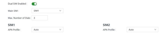
**Dual SIM enabled**: enables the dual SIM feature. EC954 supports dual card single dial to improve network reliability. Two SIM cards need to be inserted into the device. After enabling this function, if the SIM card 1 fails to dial due to arrears, it will automatically switch to the SIM card 2 for dialing. The default is off.
