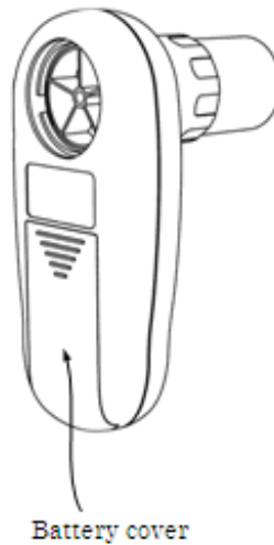
Figure3-1 MSA1000 battery assemble
