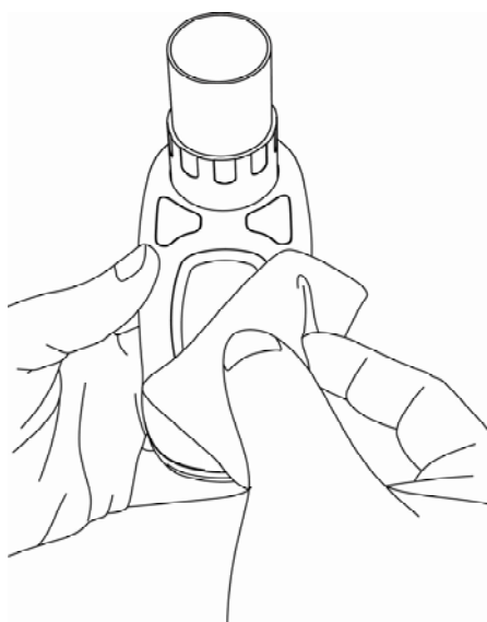
Figure3-4 cleaning to main unit
