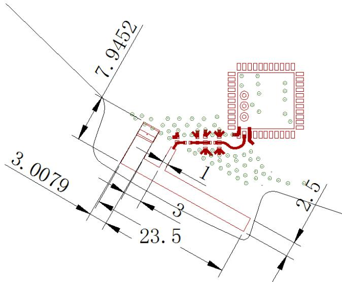
4) PCB thickness is 1.5mm, Copper-Layer 6, Antenna is Layer1;
