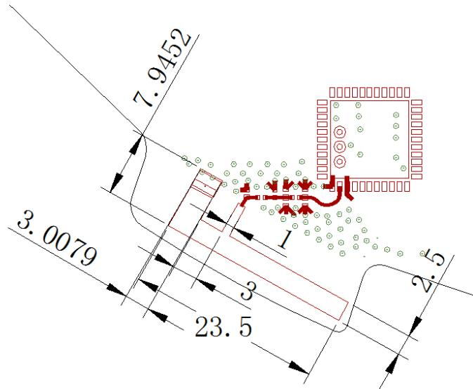
d) PCB thickness is 1.5mm, Copper-Layer 6, Antenna is Layer1;
