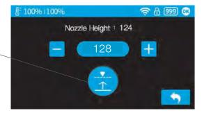
During nozzle height detection, the print head nozzle will touch the thin metal sheet on the detector to make meas- urement.
