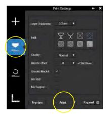
Click "Print" to start transferring the model data to the printer. Once the transmission finishes, the software will prompt the estimated printing time and material consumption. At this time, the printer can be disconnected from the computer.
