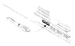
Insert USB cable into the down stream port of the PC (or) this product. Make sure that it goes all the way into the socket and is firmly connected.
