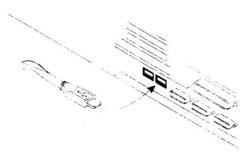
Insert USB cable into the down stream port of the PC (or) this product. Make sure that it goes all the way into the socket and is firmly connected.
