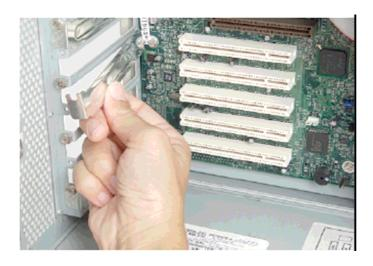
2.5 Push the Card firmly into the PCI slot that you have chosen. Apply pressure as needed until the connector is fully seated.
